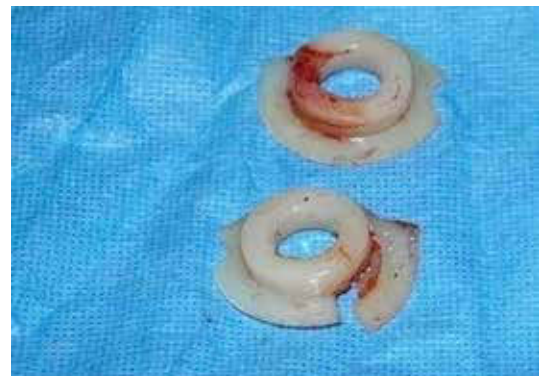
Postoperative radiographs from March 2014 (left and center); 35-year-old polyethylene bearings after removal
