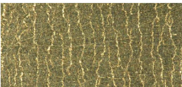
Surface treated with LINK PorEx® after bending test No delamination of layer, 100x
