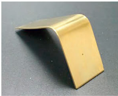
Adhesion strength of LINK PorEx® – bending test
