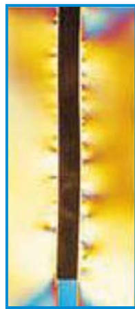
S-shaped stems result in even stress distribution
