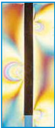
Straight stems produce stress risers in the anatomically S-shaped medullary canal
